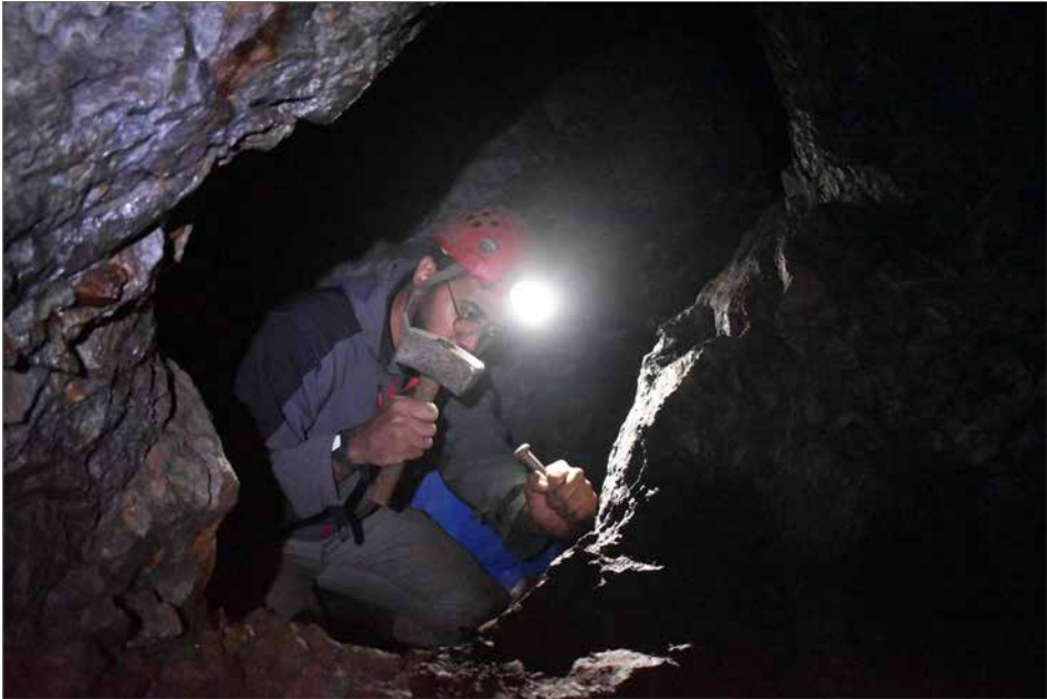
Figure 3. Mining with tools on a shale working face in the Lauqueille mine.
