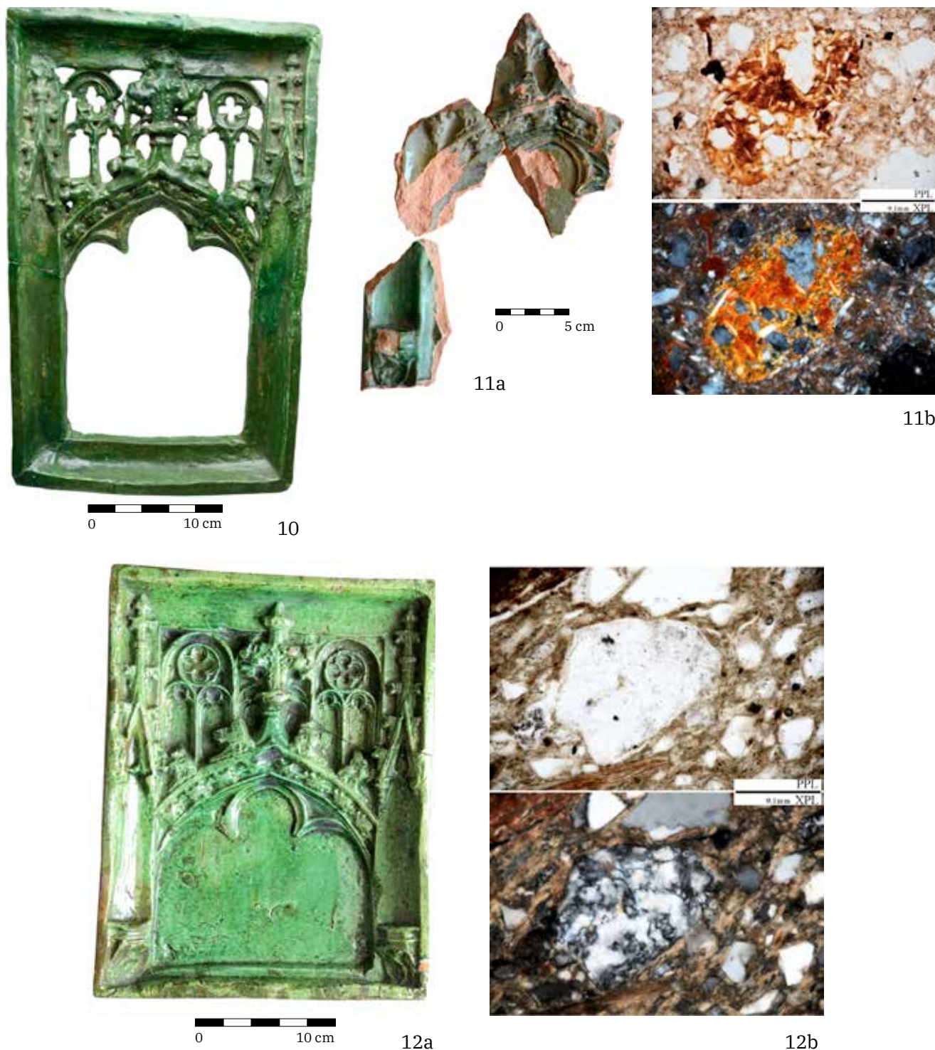
Fig. 3. Gothic architecture in square format of the frontal heating panel, type 3 after I. Holl. 1 – Budapest, stove tile of type 3 in castle exhibition; 2a – Brno, Petrov No. 2 (R4); 2b – fragment of rubified biotite in the microstructure of the ceramic shard, PPL, XPL; 3 – Brno, Jakubská St. No. 7; 4 – Brno, Milady Horákové St.; 5a – Lipnice, castle; 5b – kyanite fragment in the microstructure of the ceramic shard, PPL, XPL; 6a – Lipnice, castle, King David as a prophet (R22); 6b – claystone and quartzite fragments in the microstructure of the ceramic shard, PPL, XPL; 7 – Lipnice, castle, St. Peter; 8 – Lipnice, castle, St. Christopher; 9 – Lipnice, castle, St. Agnes; 10 – Lichnice, castle; 11a – Helfštýn, castle (R33); 11b – greywacke sandstone fragments in the microstructure of the ceramic shard, PPL, XPL; 12a – Olomouc? (R30); 12b – siliceous rock fragment in the microstructure of the ceramic shard, PPL, XPL.
