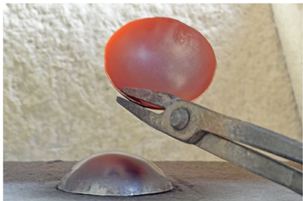
D - Annealing the hemispheres to relax the microstructure
