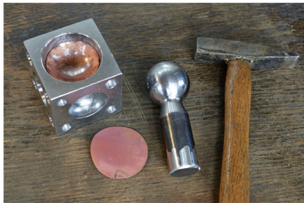
B - Forging into hemispheres in a swage block
