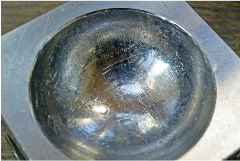
L - Deformed surface of swage block by cold forging sheet iron
