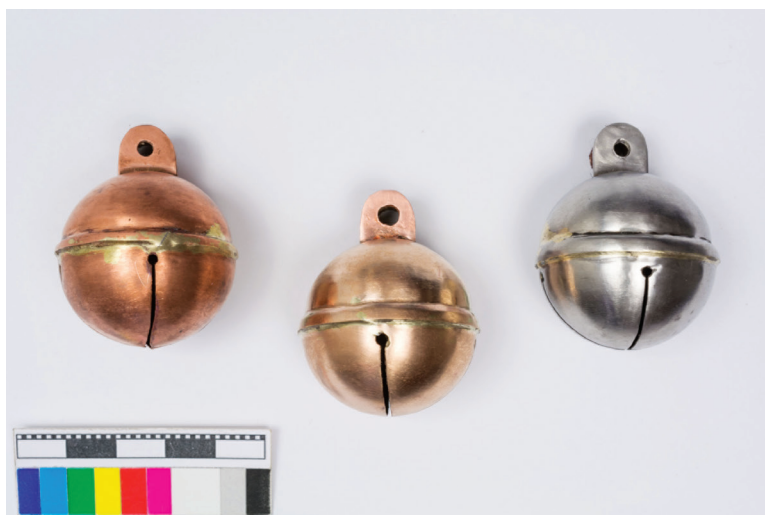
I - Finished pellet bells made from two soldered halves copper - bronze - iron
