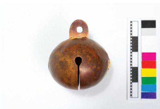
K - Pellet bell forged from one piece of sheet
