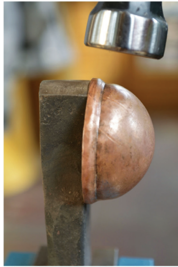
F - Levelling the outer end of the edge
