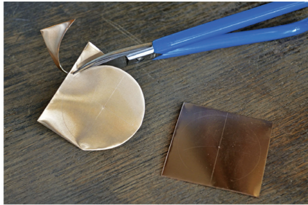
A - Cutting out the sheet metal disks
